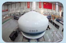
The test platform of C919, called "iron bird," was launched by Commercial Aircraft Corp of China in Shanghai's Baoshan District. The platform undertook 60,000 hours of life verification for the C919.
